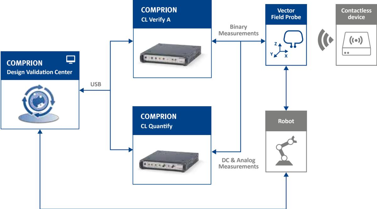
Figure 1: Setup for 3D vector field scan with Design Validation Center installed on host PC, CL Verify A, CL Quantify, and Vector Field Probe
