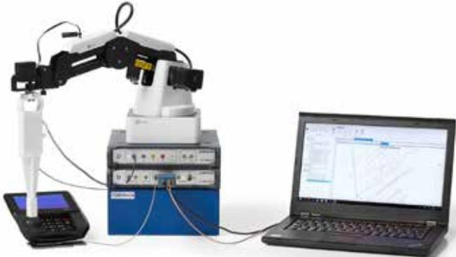
Figure 4: Setup with robot for automated measurements
