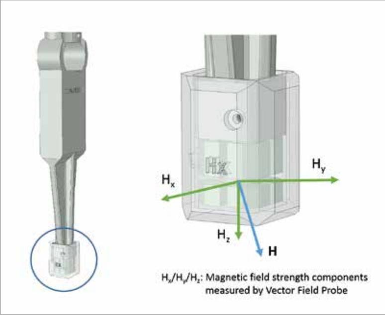
Figure 2: Measurement of magnetic field vector H with Vector Field Probe
