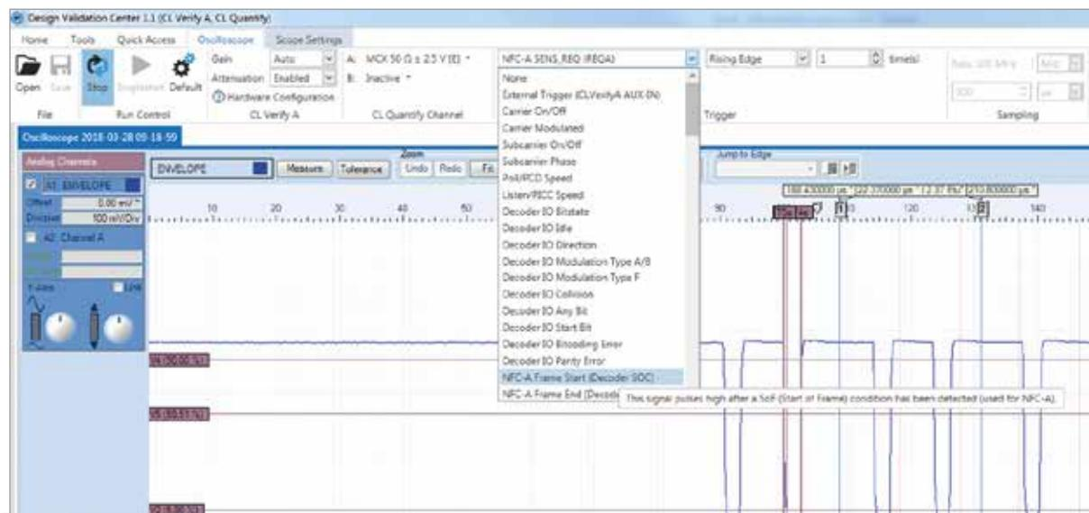
Figure 7: Convenient trigger selection provided by the integrated NFC oscilloscope
