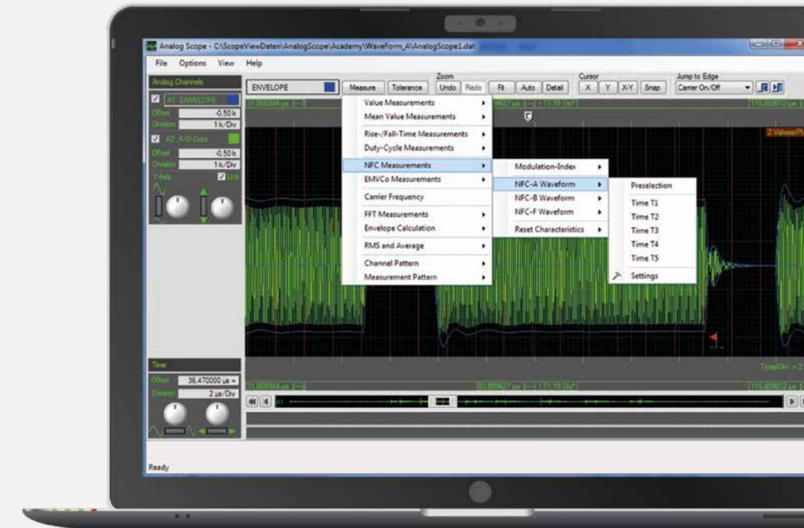
Figure 8: With a single mouse click, you can carry out predefined quick measurements. This function provides you with information on the waveform characteristics such as the modulation index and the frequency spectrum. It also supports you with detailed comments explaining why a test has failed.
