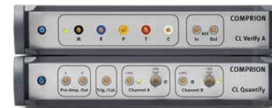
COMPRION hardware modules for contactless pre-conformance testing
